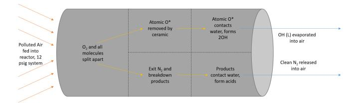
Hundreds/thousands of these ceramic cells can be skid mounted for deployment on land or ships. On a ship, the oxide gas is piped to spargers (bubbled) in the water. This oxide forms "doublet" hydroxyl: O\* +H2O = 2OH\*. Then the magic begins rapidly as the oxide and hydroxyl are infinitely soluble in water.
